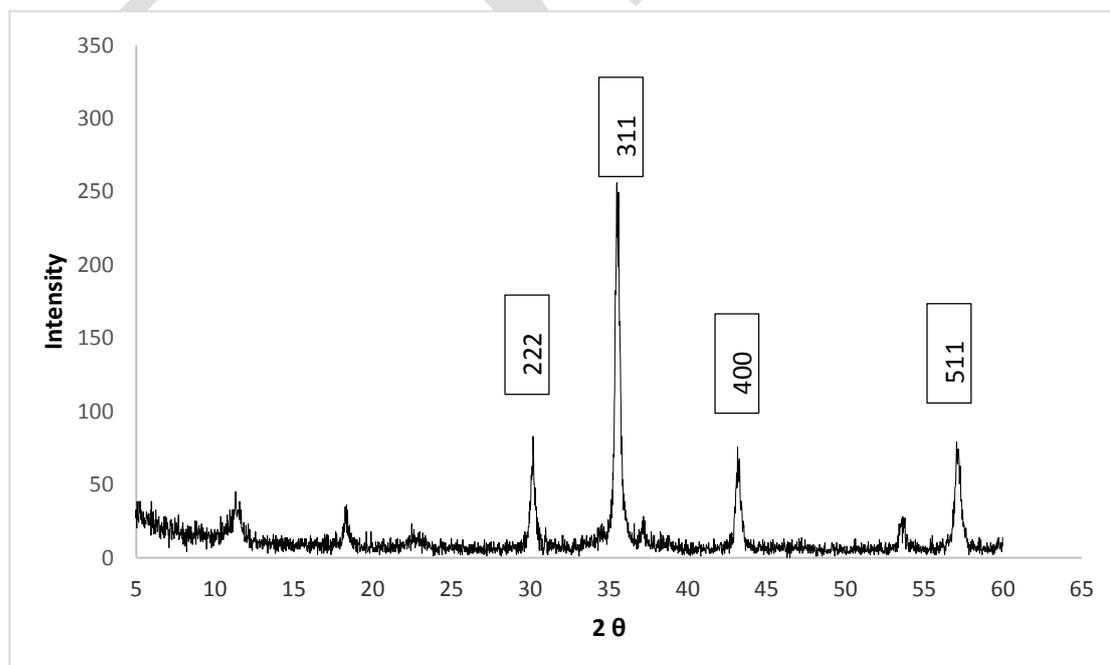
**Fig. 15 XRD pattern of prepared nickel ferrite**
