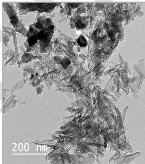
**Fig. 2.** HRTEM micrographs of NMHAp
