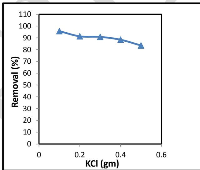
**Fig. 7.** Effect of salinity on the removal percent % of Cd (II) on NMHAp at 25°C.
