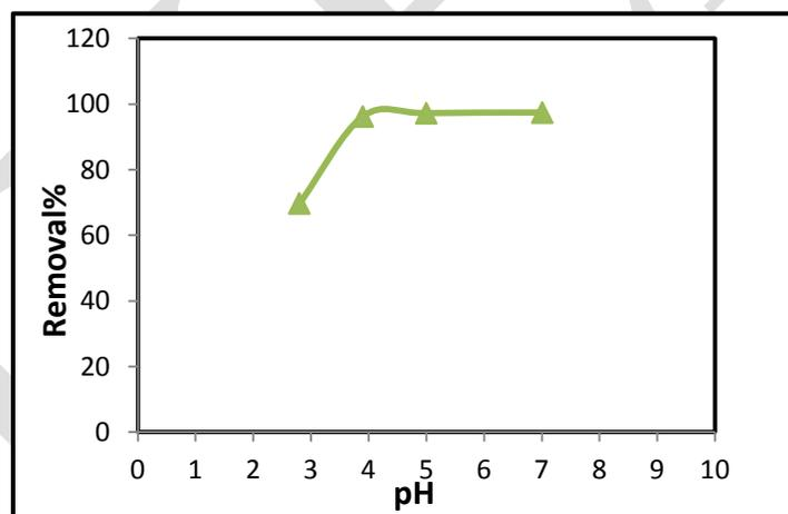
**Fig. 4.** Effect of pH on the removal percent of Cd (II) on NMHAp at 25°C.
