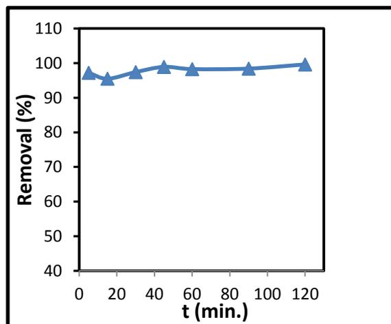
**Fig. 5.** Effect of contact time on the removal percent of Cd (II) on NMHAp at 25°C.
