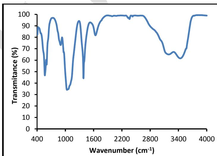
**Fig. 1.** FTIR spectra of nanomagnetic-hydroxyapatite
