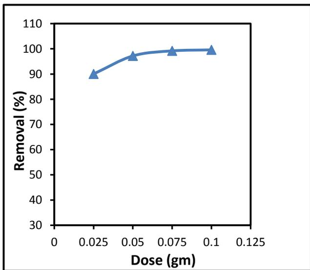
**Fig. 6.** Effect of adsorbent dosage on the removal percent % of Cd (II) on NMHAp at 25°C.
