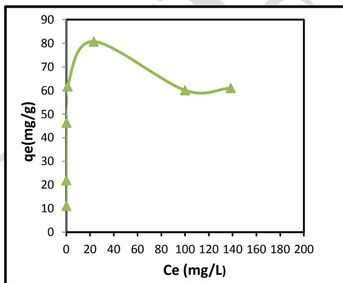
**Fig. 3.** Effect of initial metal ion concentration on the uptake of Cd (II) using NMHAp as adsorbent at 25°C.
